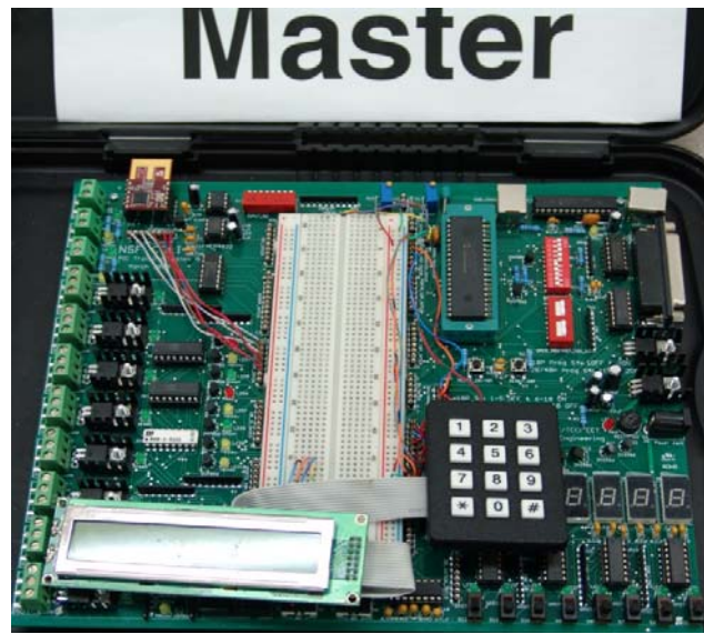
Photo 1. Master System Board
